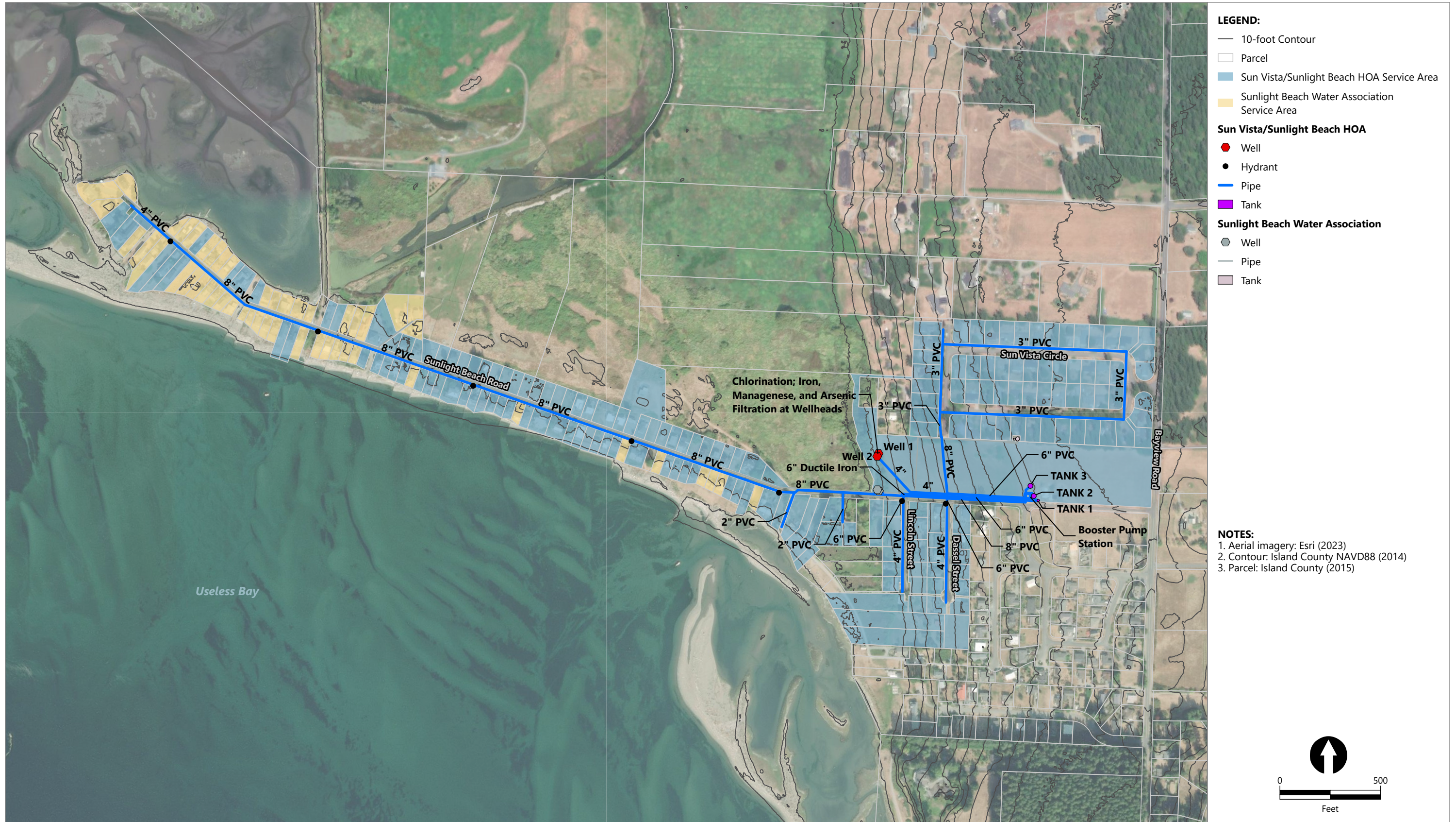
Figure 2 Existing Water System – Sun Vista/Sunlight Beach Homeowner’s Association Sun Vista/Sunlight Beach Water Consolidation Feasibility Study
